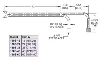
The Series 160S "S" Type Stainless Steel Pitot Tubes are designed specifically for flow measurement of dirty, particulate laden air or gas streams typical in smoke stack and other environmental testing. Total and static pressure tubes are precisely aligned and welded together every 6 inches for maximum accuracy, strength, and long term durability. Permanent mount (PM) models include a 1" welded stainless steel sleeve and adjustable compression fitting with 1" MNPT mounting threads.
